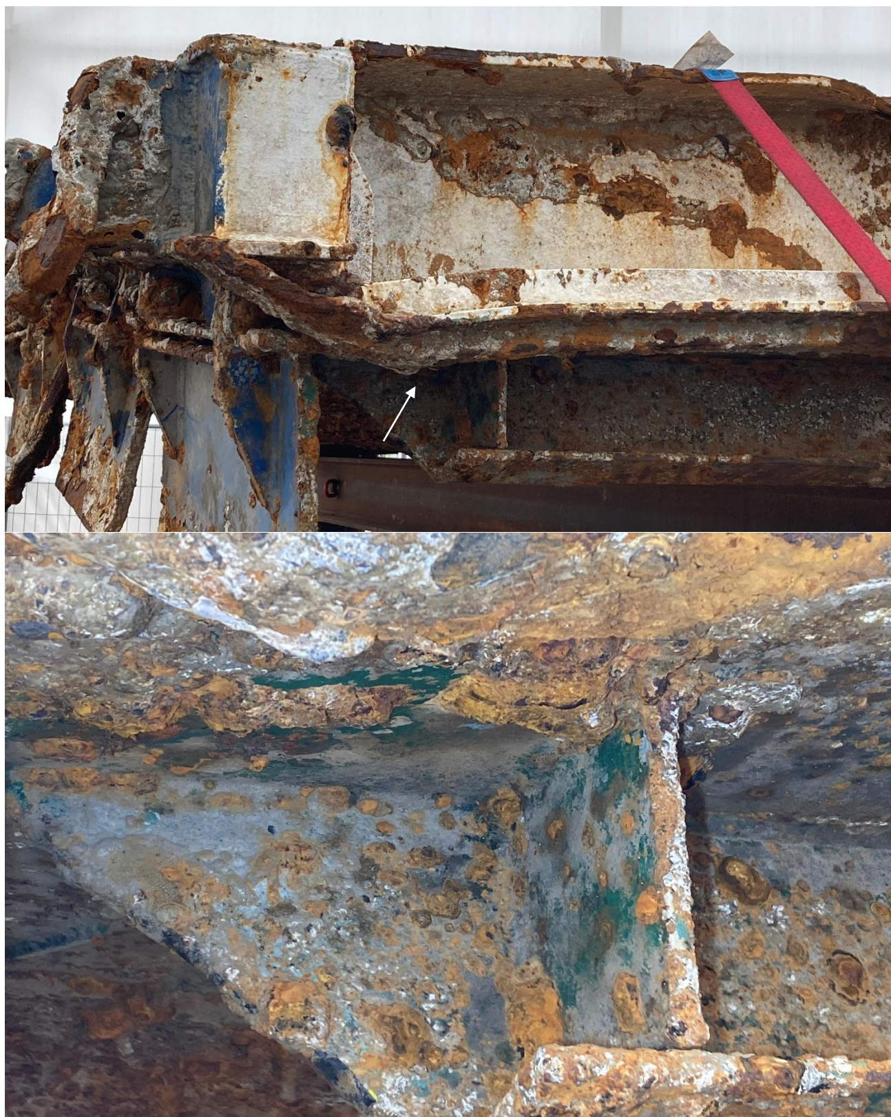
Figure 16. Port side attaching position for railing, no part of the railing remains, the weld has been somewhere below the heavily corroded area (4 in Figure 12).
