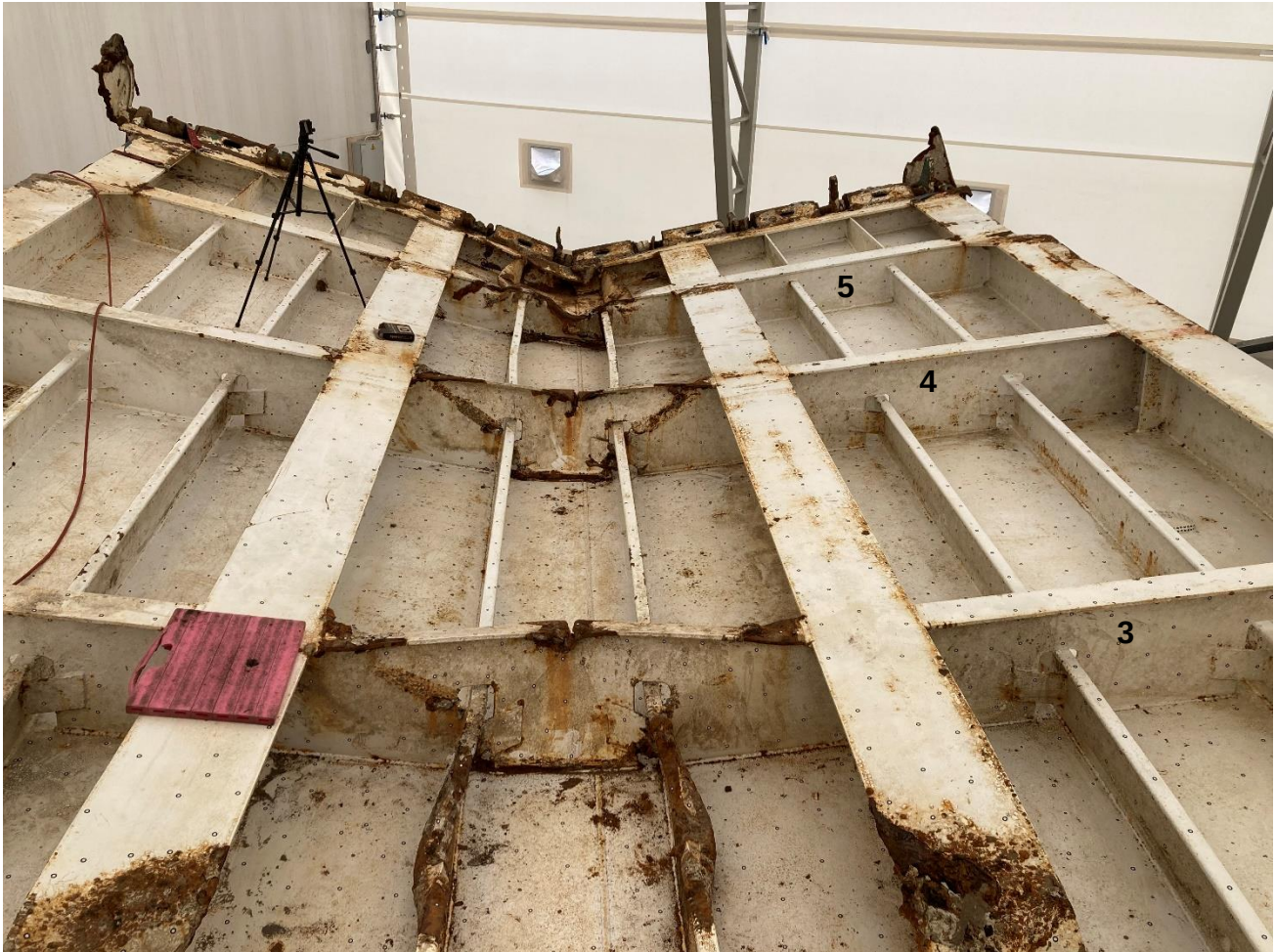
Figure 7. The sea side of the bow ramp seen from the hinge side, transverse beams 3, 4 and 5 marked.
