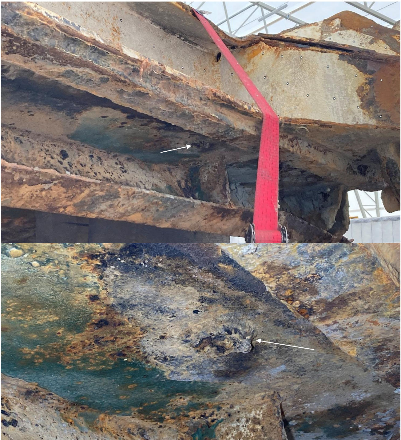
Figure 11. Starboard attaching position for railing, only the weld fillet remains on the bow ramp (3 in Figure 8).
